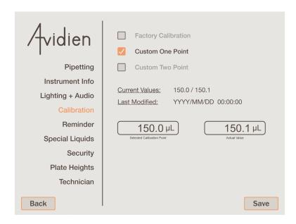
After selecting a Custom One Point calibration, the above will be displayed. Here you can enter the desired calibration value along with the subsequent actual value. This will adjust the instrument's calibration curves accordingly.
