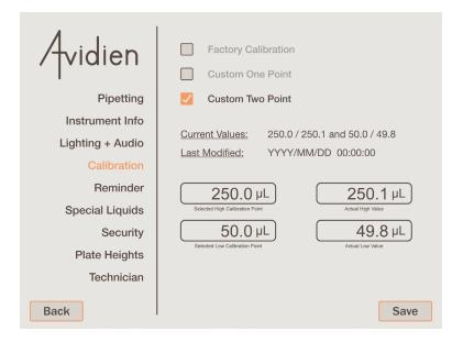
After selecting a Custom Two Point calibration, the above will be displayed. Here you can enter the desired high and low calibration values along with the subsequent actual values. This will adjust the instrument's calibration curves accordingly.
