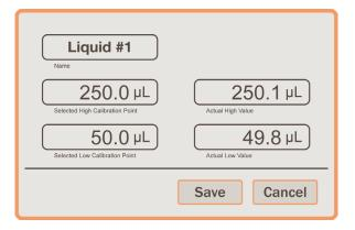
To create a new special liquid, simply press on the top row labeled <Create New>. Then, the pop-up window above will be displayed. Here you can enter in the name of the special liquid and the desired calibration values along with the subsequent actual values.
