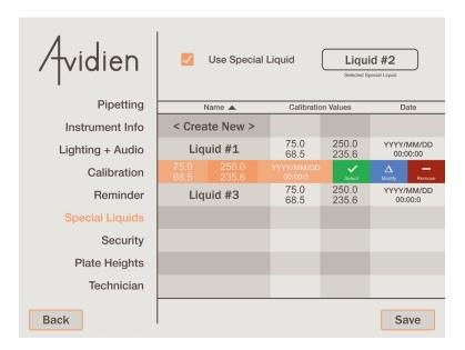
If you would like to Select, Modify or Remove a special liquid that has already been created, simply swipe that row to the left. The three corresponding buttons will be revealed. (see image above) Once you have special liquids turned on and the desired one selected, simply press the SAVE button at the bottom of the screen as usual.
