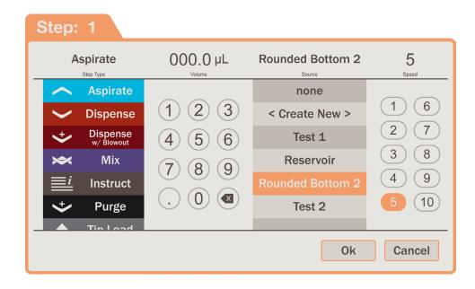
The main difference is that now you can select the type of step you would like to create. Once you have selected the step type, the rest of the pop-up window options will be displayed accordingly. In the case of the standard steps such as Aspirate, Dispense, and Mix they are identical as to what you have used before. For the other step types only available in Custom programs, each one is a bit different.
