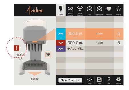
When the reminder elapses, a red exclamation point symbol will be shown next to the image of the pipettor on the main screen. (see image above) Pressing on this symbol will tell you that it is time for maintenance.
