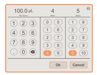
To add a mix step, press on the Add Mix step located just below the dispense step. The above pop-up window will be displayed. Here you will be able to edit the mix volume, the total number of mixes, and the speed.
