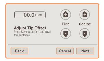
After pressing NEXT, the above pop-up will be displayed. While continuing to hold the tips down, press the FINE and COARSE adjustment buttons until you have reached the desired distance between the tips and the bottom of the container. Then, press NEXT and the pop-up below will be displayed.
