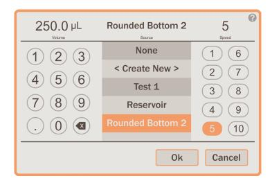
Within this pop-up window, you can edit the volume, select the desired container, and edit the speed. To edit the volume, simply use the keypad to enter in the desired volume in  $\mu$ L. From the list of containers, you can select any of the pre-existing containers, select none, or choose to create a new one. For more details on creating a new container, see Section 4.6 below. Note that this is the container that liquid will be aspirated from.
